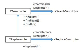
Figure 2. The XReplaceable and XSearchable Interfaces.
